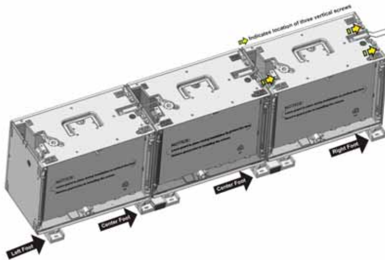
Figure 2-9 Assemble Final Tile in First Row
